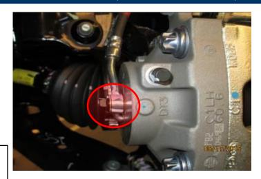
4. Remove caliper mounting bolts.
